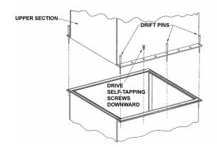
Figure 12 - Mating Upper Section to Basin Section
