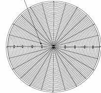
Figure 17 - Wire Clip Spacing
