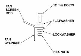
Figure 15 - Attaching Fan Screen to Cylinder
