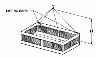
Figure 2a - Basin Section up to 6,3 m long
