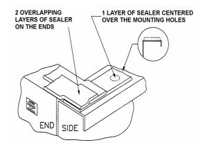
Figure 9 - Proper Sealer Tape Application
