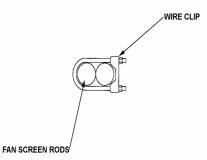
Figure 16 - Wire Clip Arrangement
