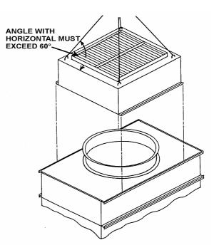
**Figure 22** - Mating Discharge Hood Damper Section to Coil/Fan Section
