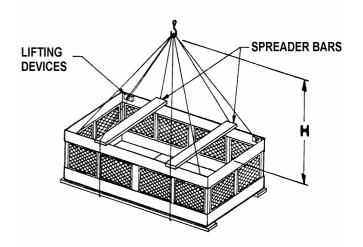
Figure 11 - Extended Lifts, Basin Section
