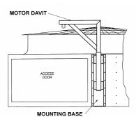
Figure 19 - Single Point Davit Arrangement
