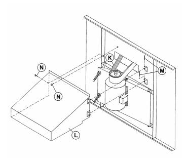
Figure 24 - Motor Guard and Powerband Belt Installation
