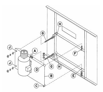
Figure 23 - External Motor Installation
