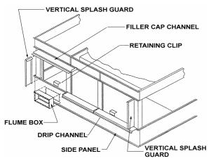
Figure 8 - Drip Channel and Splash Guards, 4,9 - 5,3 and 7,3 m wide models
