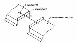
Figure 7 - Drip Channel Assembly
