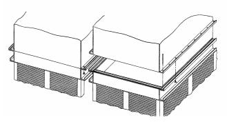
Figure 13 - Mating Upper Section to Basin Section
