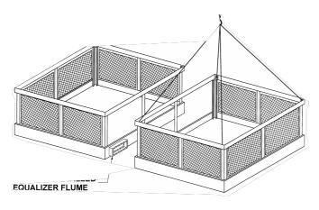
Figure 4 - Equalizer Flume Rigging Detail
