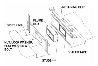
**Figure 6** - Equalizer Flume Assembly, 4,9 - 5,3 and 7,3 m wide models
