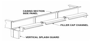
Figure 14 - Filler Cap Channel Assembly
