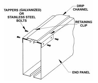
Figure 5 - Drip Channel Installation
