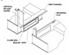
Figure 3 - Equalizer Flume Connection
