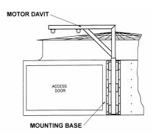
Figure 20 - Dual Point Davit Arrangement
