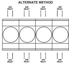
MULTIPLE UNITS PLACED END-TO-END Figure 28a
