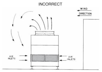
WIND EFFECT WITH TOP OF UNIT LOWER THAN TOP OF WALL
