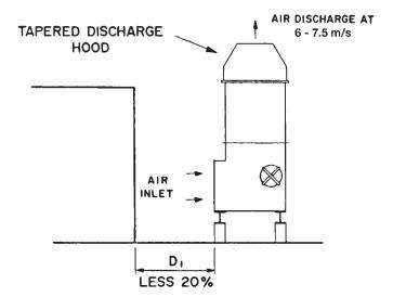
INSTALLATION WITH TAPERED DISCHARGE HOOD
