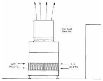
FAN DISCHARGE ELEVATED SO TOP OF UNIT IS HIGHER THAN TOP OF WALL
