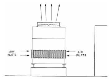
INSTALLATION ELEVATED SO TOP OF UNIT IS HIGHER THAN TOP OF WALL
