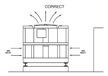
INSTALLATION FLEVATED SO TOP OF UNIT IS HIGHER THAN TOP OF WALL Figure 25
