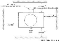
MINIMUM CLEARANCE DIMENSIONS INDUCED DRAFT COUNTERFLOW UNITS
