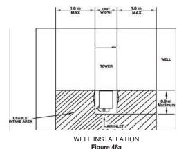
Note: Units with solid bottom panels or inlet sound attenuation, the usable well area is reduced. Only utilize the space in the front of the air inlets.
