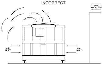
WIND EFFECT WITH TOP OF UNIT LOWER THAN TOP OF WALL Figure 24
