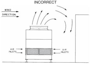
INSTALLATION WITH TOP OF UNIT LOWER THAN TOP OF WALL
