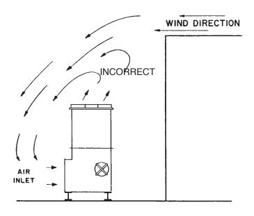
WIND EFFECT WITH TOP OF UNIT LOWER THAN TOP OF WALL
